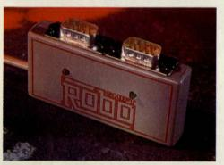
This handy little device plugs into the mouse port, and can have a mouse and joystick plugged into it. Just press fire or a mouse button to select the right device.
