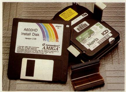
The two important components are the hard drive (seen still attached to the mounting plate) and the cable. The Install disk is nearly indispensable if the hard drive develops a fault — note the A600 Install disk is pictured. The A1200 needs the Install disk for Workbench 3.
